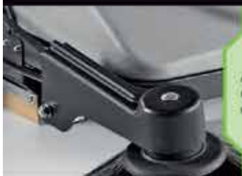
Adjustable side brush mounted on shock-absorbers
